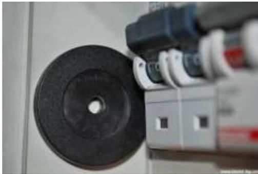
Global Tag **ON-METAL TOKKY 34** is a wall-mount rugged IP68 transponder with a 5mm central hole. It is available in LF, HF (both ISO14443 and ISO15693), and also NFC.
