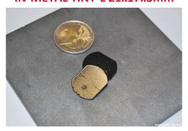
Global Tag **IN-METAL TINY-L** is in-metal or on-metal UHF tag, with high performance for indoor and outdoor environments. The reading distance can reach up to 350cm with long range controller RFID UHF with 2W ERP. Generally is made with 3M adhesive for an easy attached way. Available as option magnet for on-metal attaches / detaches solution.
