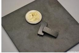
Global Tag **IN-METAL TINY-XL** is in-metal or on-metal UHF tag, with high performance (reading distance near to 400cm). It's designed for indoor and outdoor environments and it is the best solution if you need to integrate transponder into a longer but not thick metal objects for applications as IT asset management, maintenance of tools and machinery. As option we can propose 3M adhesive and printing options serial number and printing logo, TID and EPC encoding.
