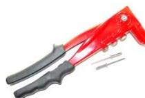
**Note:** Screw or Pop Rivet are recommended to be used in every application that includes risk for high mechanical stress or low temperature during tag fixing with adhesive.
