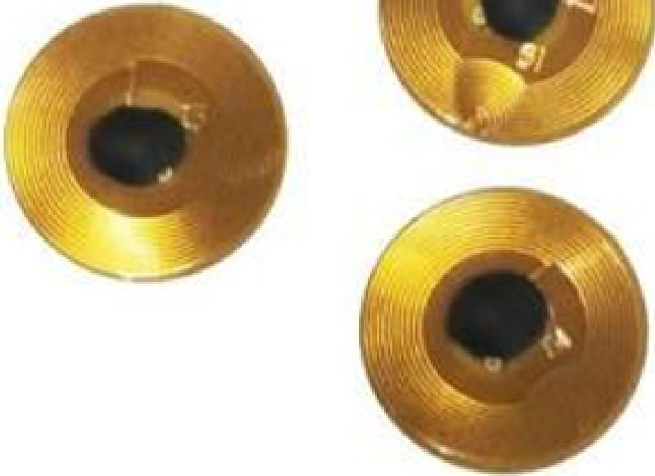
Ultra-compact and flexible RFID tag with NTAG213 chip. Ideal for curved or embedded applications in jewelry, cosmetics, and small electronics.
