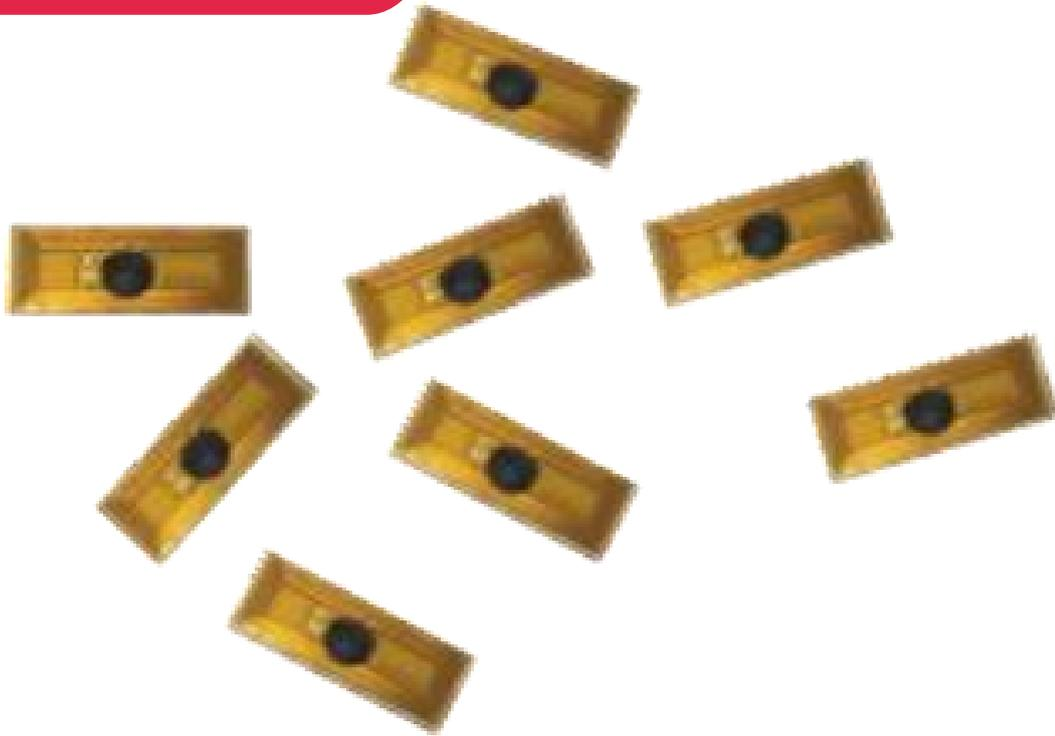
Slim rectangular tag with NTAG213 chip and up to 20 mm read range. Perfect for smart packaging, electronics, and item-level tracking.
