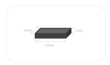
**Mounting System:** for in-metal solution need to make hole 28x13mm with 4mm depth.
