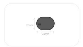
Mounting System: for in-metal solution need to make hole 25mm diameter with 4mm depth.
