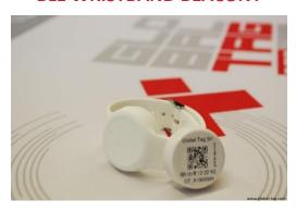
Global Tag **WRISTBAND BEACONY** is a wearable BLE Beacon, which meets the BT 4.2 protocol. Designed for hospital and healthcare applications, it can be used as a reusable wristband or a disposable bracelet, thanks to the optional anti-removal clip, which prevents the removal of the device. It is based on the basic unit DISK BEACONY, keeping its main features.
